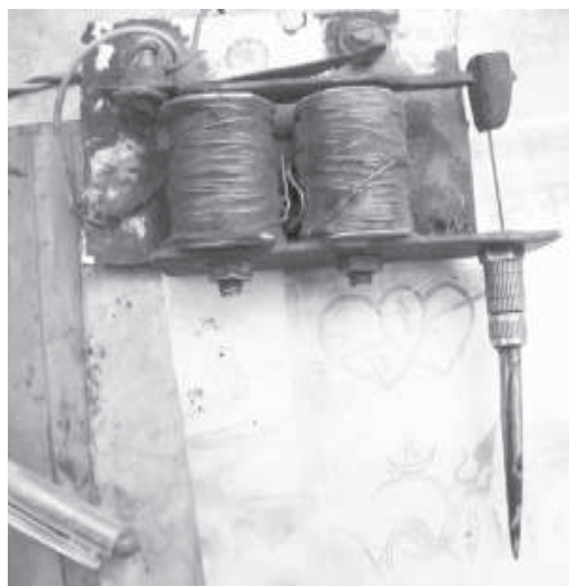
Image: 4 A battery operated tattoo making machine
